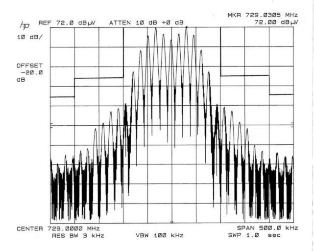
2.1051 Spurious emissions at antenna terminals(conducted):
