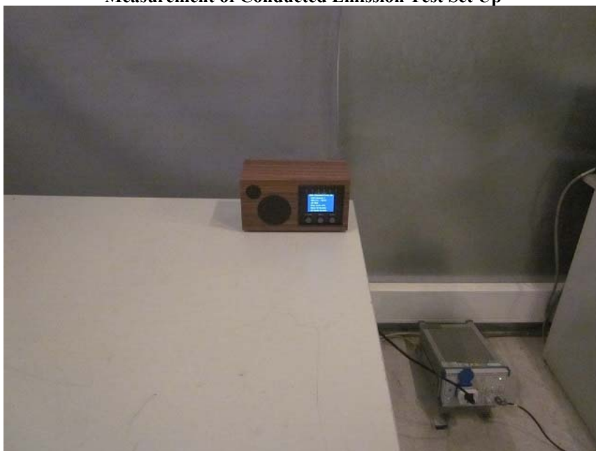
Measurement of Conducted Emission Test Set Up
