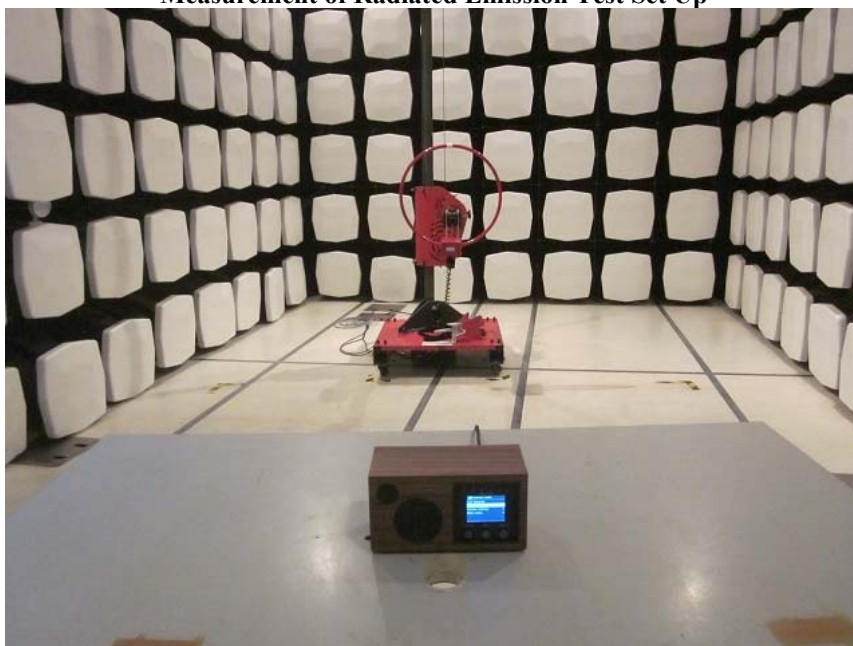
Measurement of Radiated Emission Test Set Up
