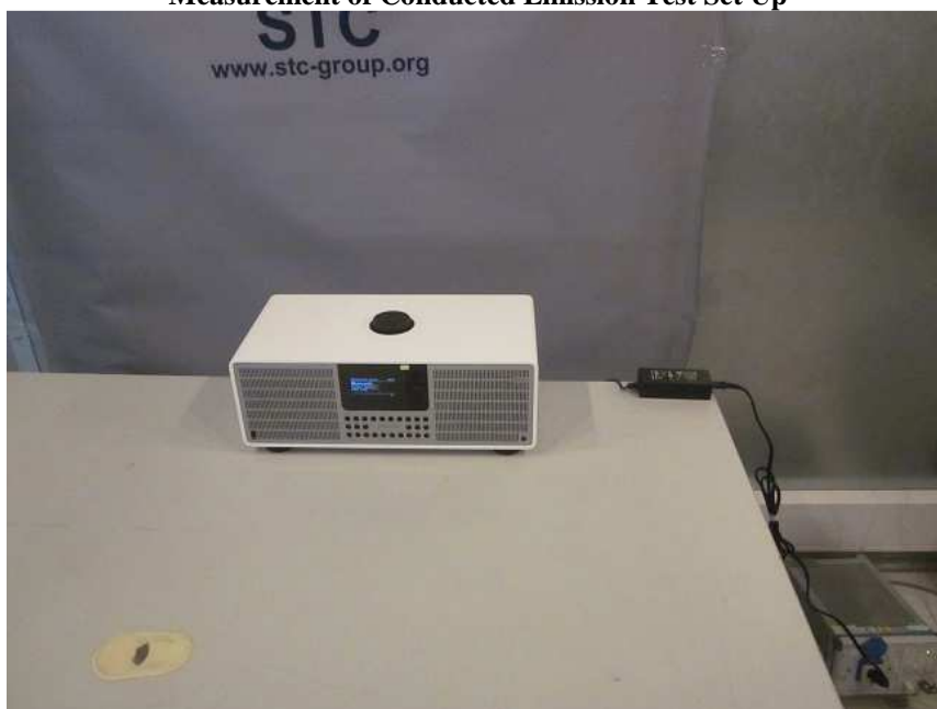
Measurement of Conducted Emission Test Set Up
