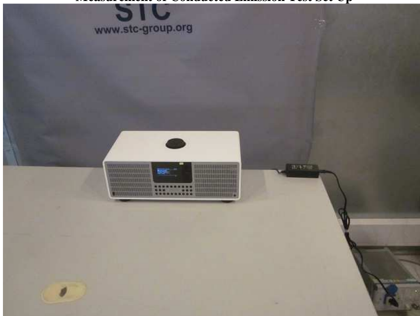
Measurement of Conducted Emission Test Set Up
