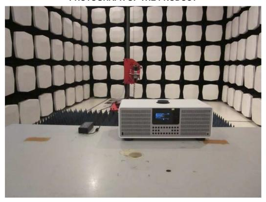
MEASUREMENT OF CONDUCTED EMISSION TEST SET UP
