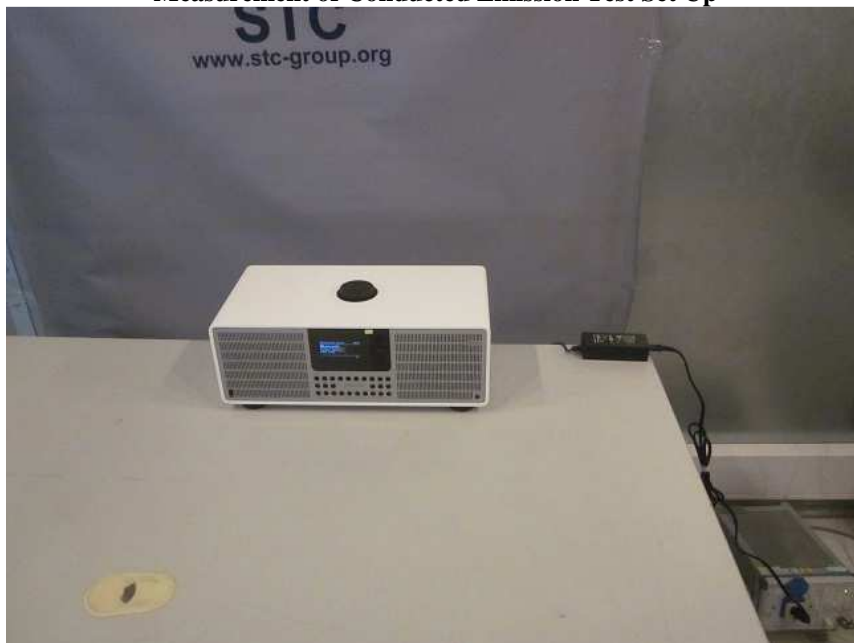
Measurement of Conducted Emission Test Set Up
