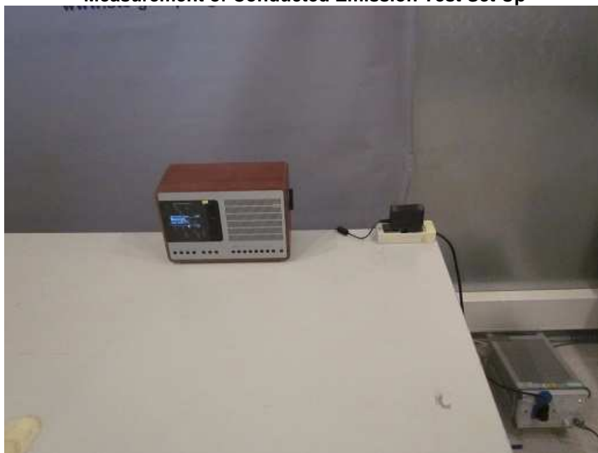
Measurement of Conducted Emission Test Set Up
