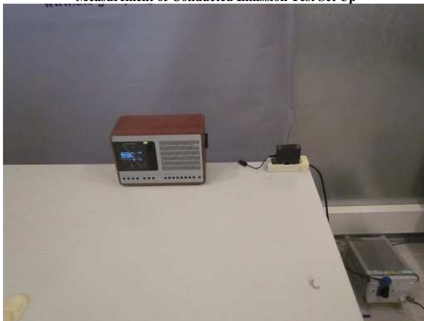
Measurement of Conducted Emission Test Set Up
