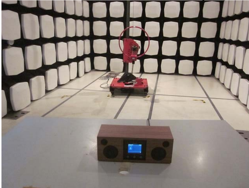
Measurement of Radiated Emission Test Set Up
