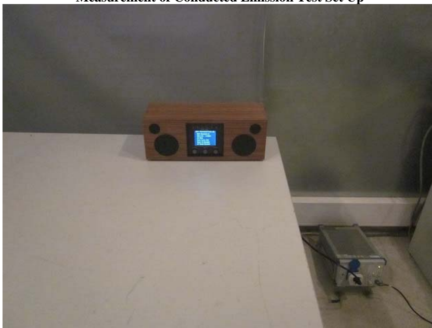
Measurement of Conducted Emission Test Set Up
