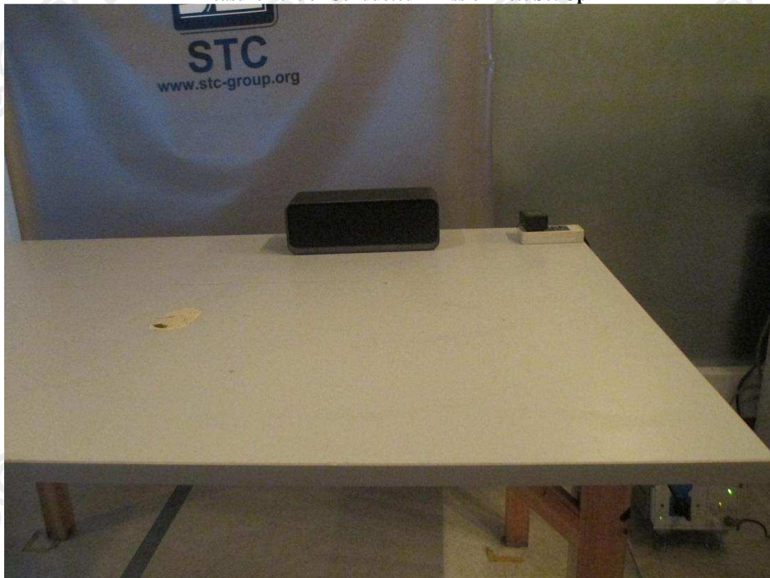
Measurement of Conducted Emission Test Set Up
