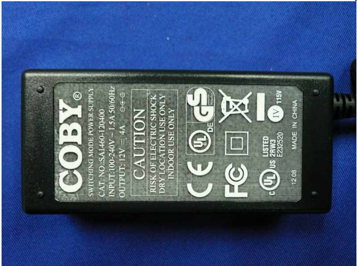
Figure 26 Switch Mode Power Supply
