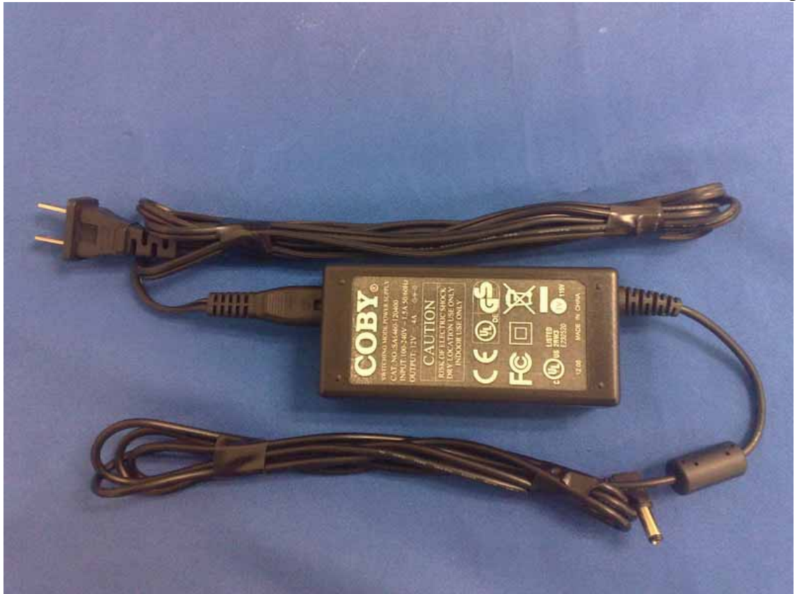
Figure 25 Switch Mode Power Supply
