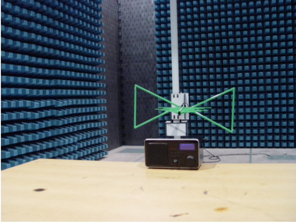
Photo 2 Radaited Emission Test
