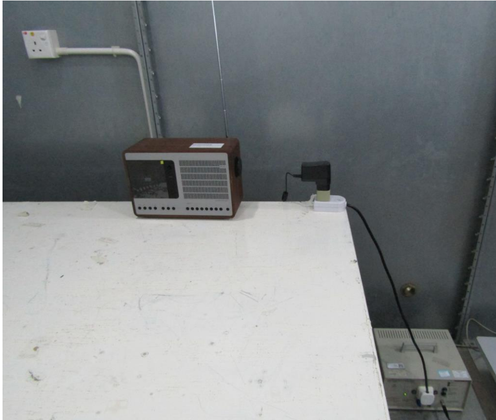
Measurement of Conducted Emission Test Set Up
