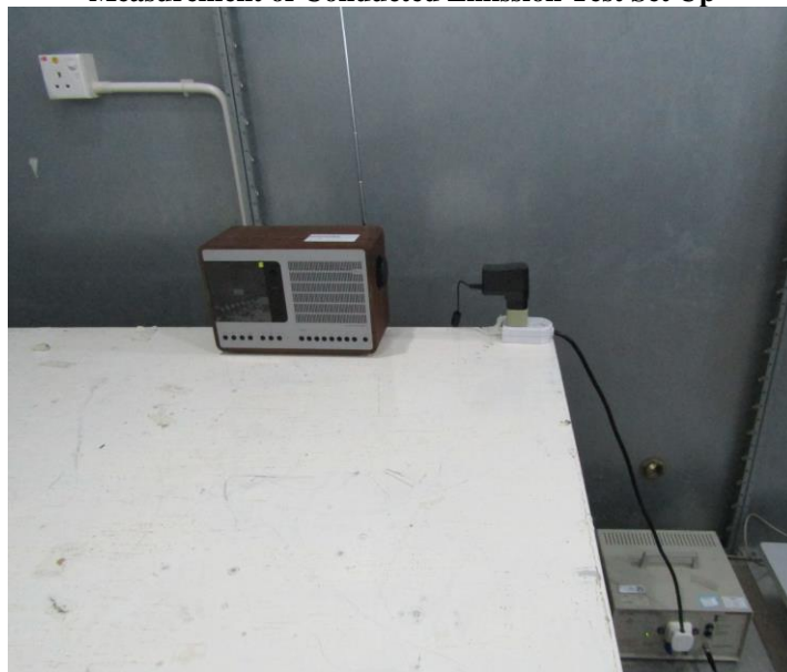
Measurement of Conducted Emission Test Set Up
