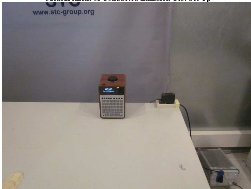
Measurement of Conducted Emission Test Set Up
