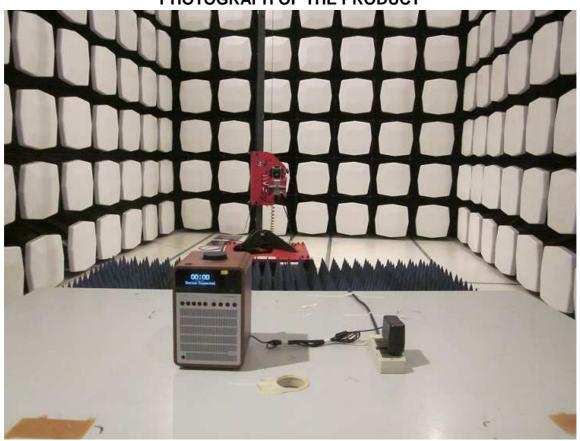
**MEASUREMENT OF CONDUCTED EMISSION TEST SET UP**
