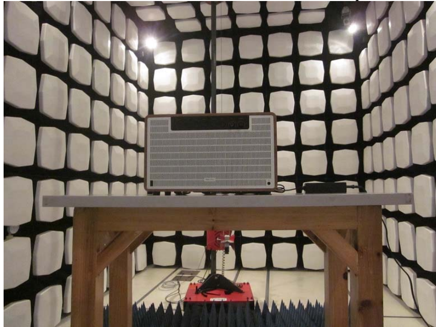
Measurement of Radiated Emission Test Set Up
