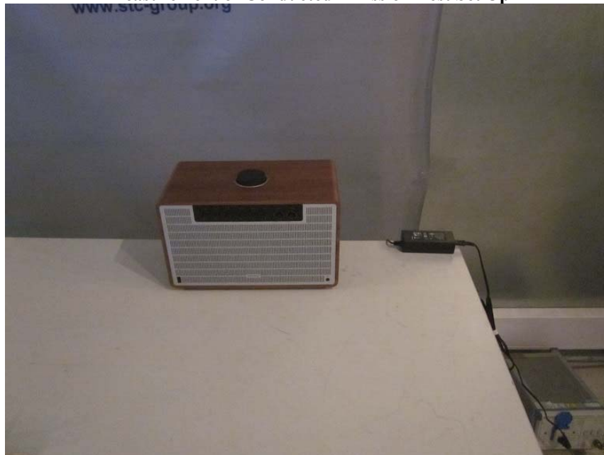
Measurement of Conducted Emission Test Set Up
