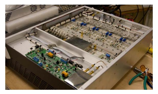
One of two identical amplifier units which operate in parallel.
