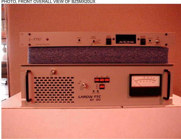
APPLICATION FOR FCC CERTIFICATION BZ5MX20UX HETERODYNE PROCESSOR INPUT 20 WATT UHF TRANSLATOR
