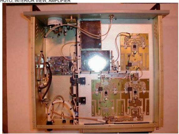
APPLICATION FOR FCC CERTIFICATION BZ5MX100UX HETERODYNE PROCESSOR INPUT 100 WATT UHF TRANSLATOR
