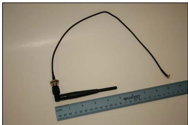
Antenna "A" - Base Station Antenna (2X): Nearson 2.4GHz Right Angle Antenna Model 181 (2dBi gain)
