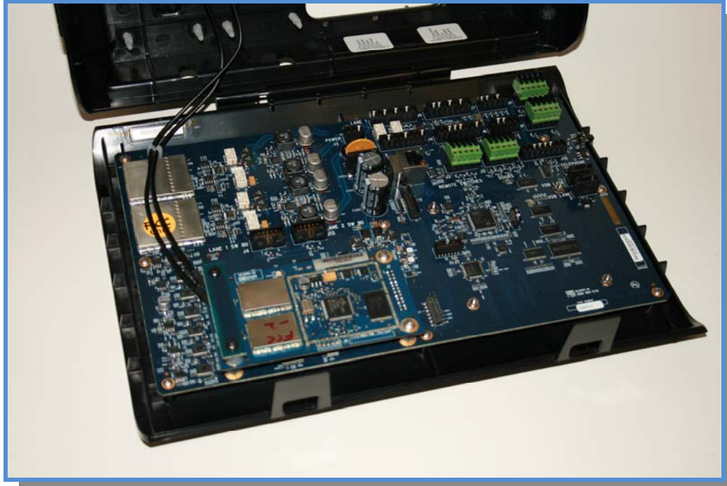
The EUT installed inside the System 6100 Wireless Base Station. The base station uses a eUrasia Power AC adapter, Model CP-8026 with serial# 08470295.
