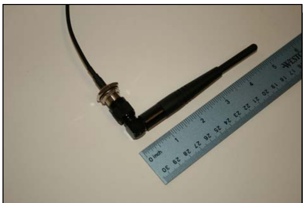
Antenna "A" - Base Station Antenna (2X): Nearson 2.4GHz Right Angle Antenna Model 181 (2dBi gain)
