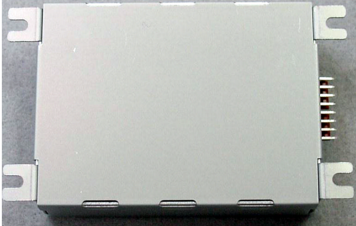
RX MODULE BOTTOM WITH SHIELD FILE: RX MODULE BOTTOM WITH SHIELD.JPG
