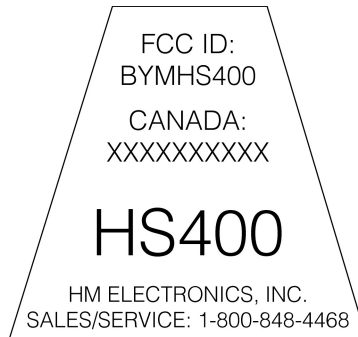
Figure 1 HS400 FCC ID Label. The Part 15 compliance statement does not appear on product, but rather is in the product manual.
