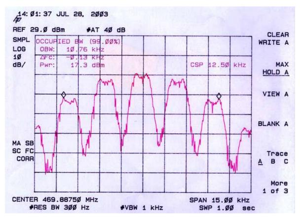
Figure 1 COM400 Modulated with 2500Hz + 16 dB
