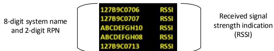
Figure 3-4 An unconnected beltpack site survey screen
