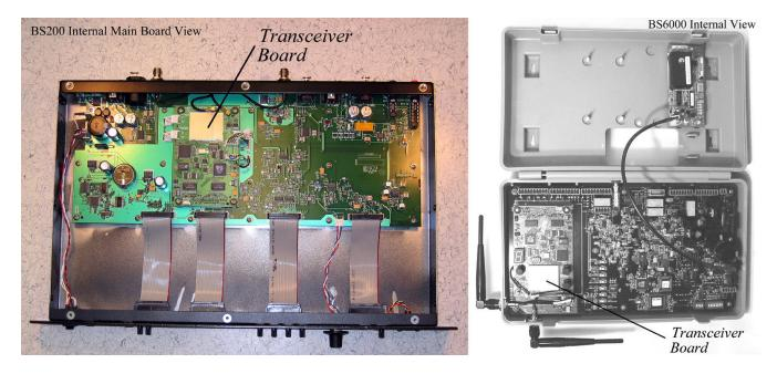
The user operable switches and indicators have been moved to the front panel in the BS200. All RF frequency components remain unchanged.
