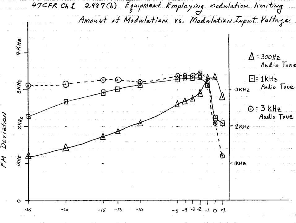
Audio Input Level in dBV Note: -20 dBV is nominal level OdBV is max level
