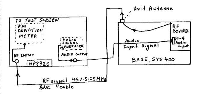
Tested Per EIA Standard EIA-TIA-603 poura 2,2,3 Methods of Measurement for Transmitters Modulation Limiting The BASE400 Base-Station is being type accepted under the rules of FCC 90.217. Therefore, the data provided is for information purposes only and no limits are required to be met.
