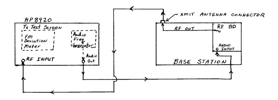
Tested Per EIA standard EIA-TIA-603 para 2,2,6 Methods of Measurement for Transmitters Andio Frequency Response,
