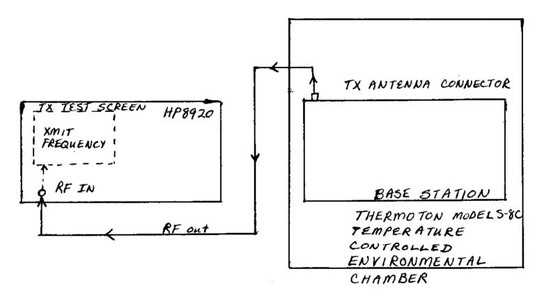
Tested per EIA standard EIA - TIA-603 para. 2,2,2 Methods of Measurement for Transmitters Carrier Frequency Stability
