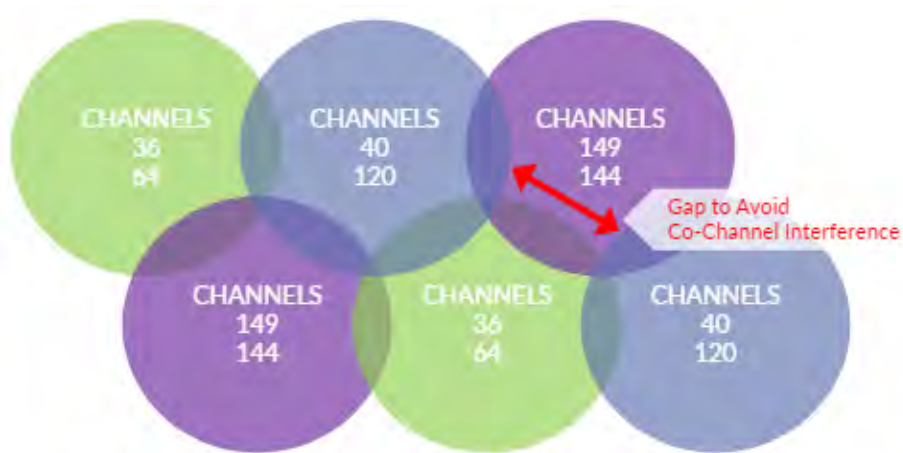
Use of 3 Zones for Overlapping Coverage to build a roaming system
