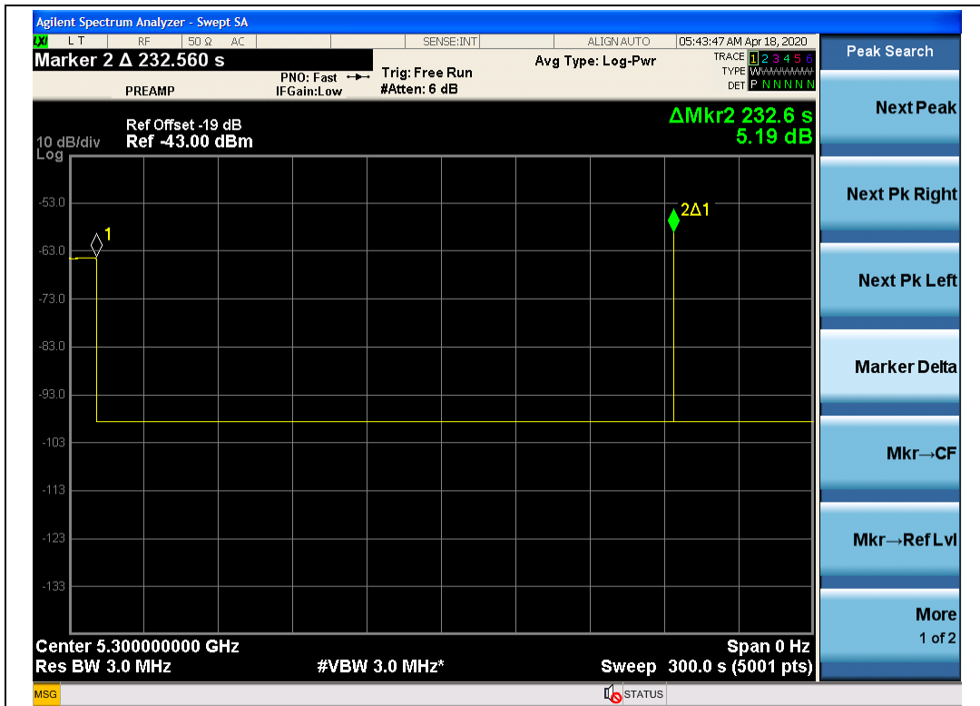
Radar at end of CAC -5300MHz
