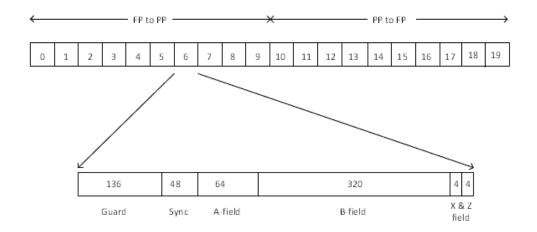
1 frame = 20 slot Crystal freq = 10.368 Mhz
