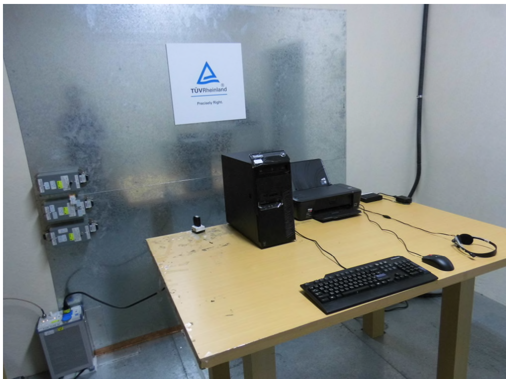
Photograph 6: Set-up for for Mains Conducted testing Front
