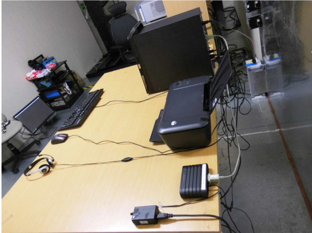
Photograph 5: Set-up for for Mains Conducted testing Back
