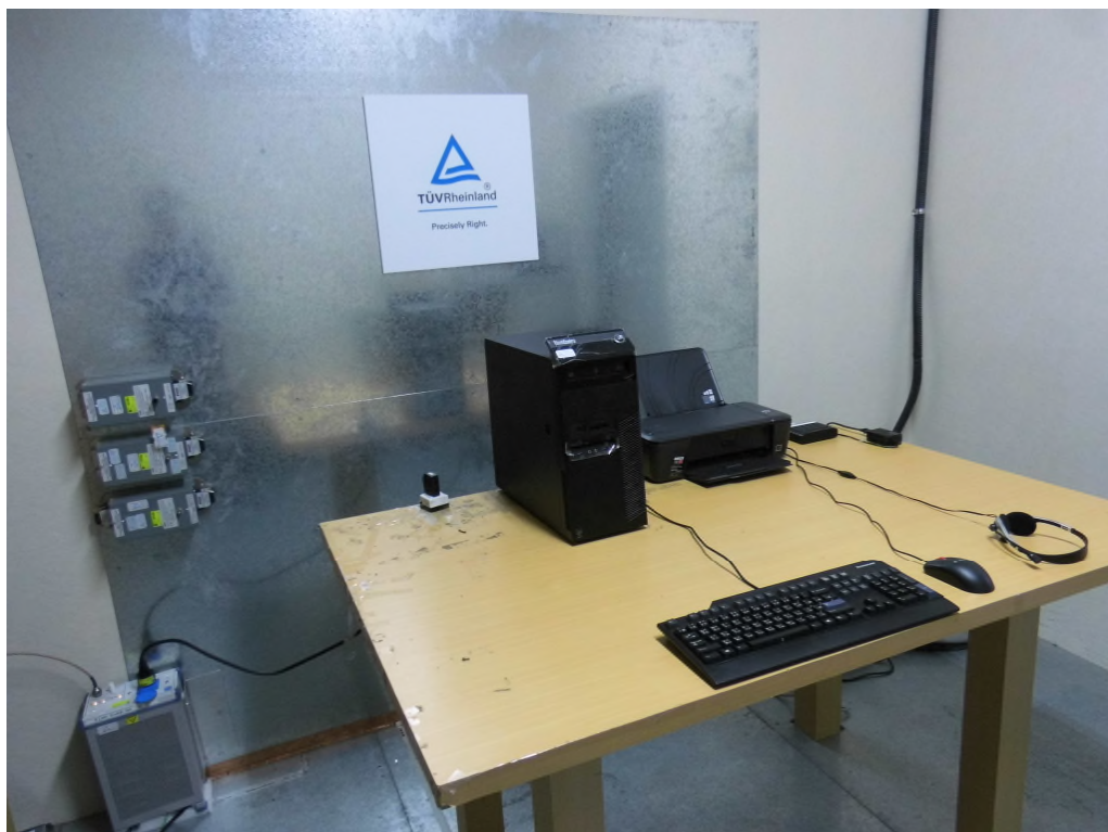
Photograph 6: Set-up for for Mains Conducted testing Front
