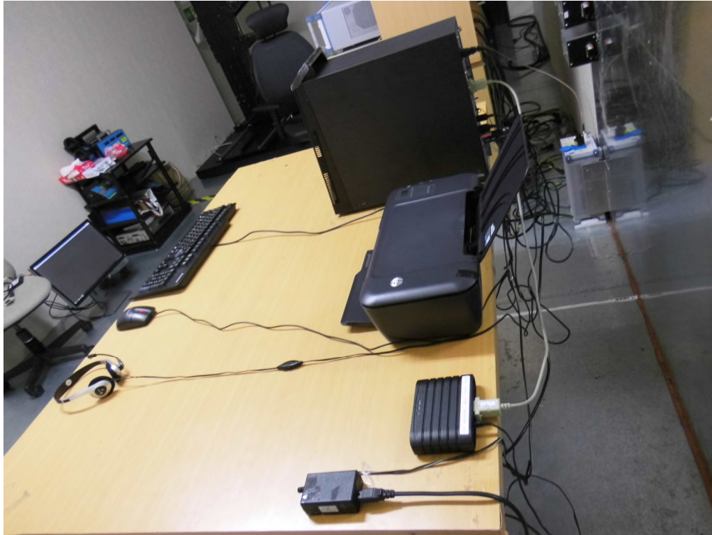
Photograph 5: Set-up for for Mains Conducted testing Back
