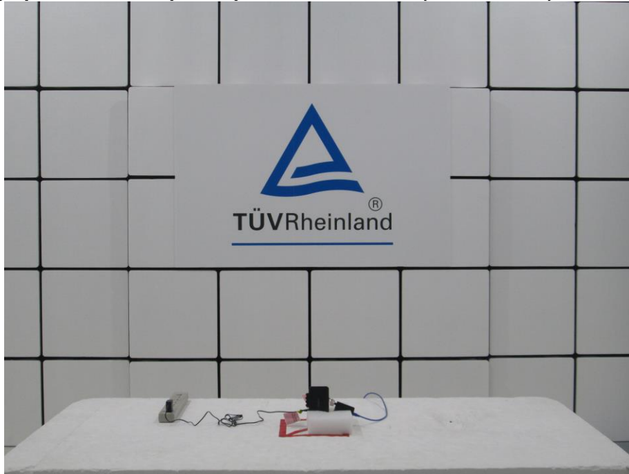
Photograph 2: Test Setup for Spurious Emissions (Front View 2)
