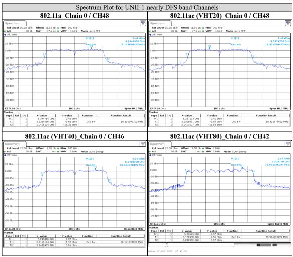
Note: The observed T2 is all <5250 MHz, so UNII-1 band channels which in nearly DFS band no need for DFS function.
