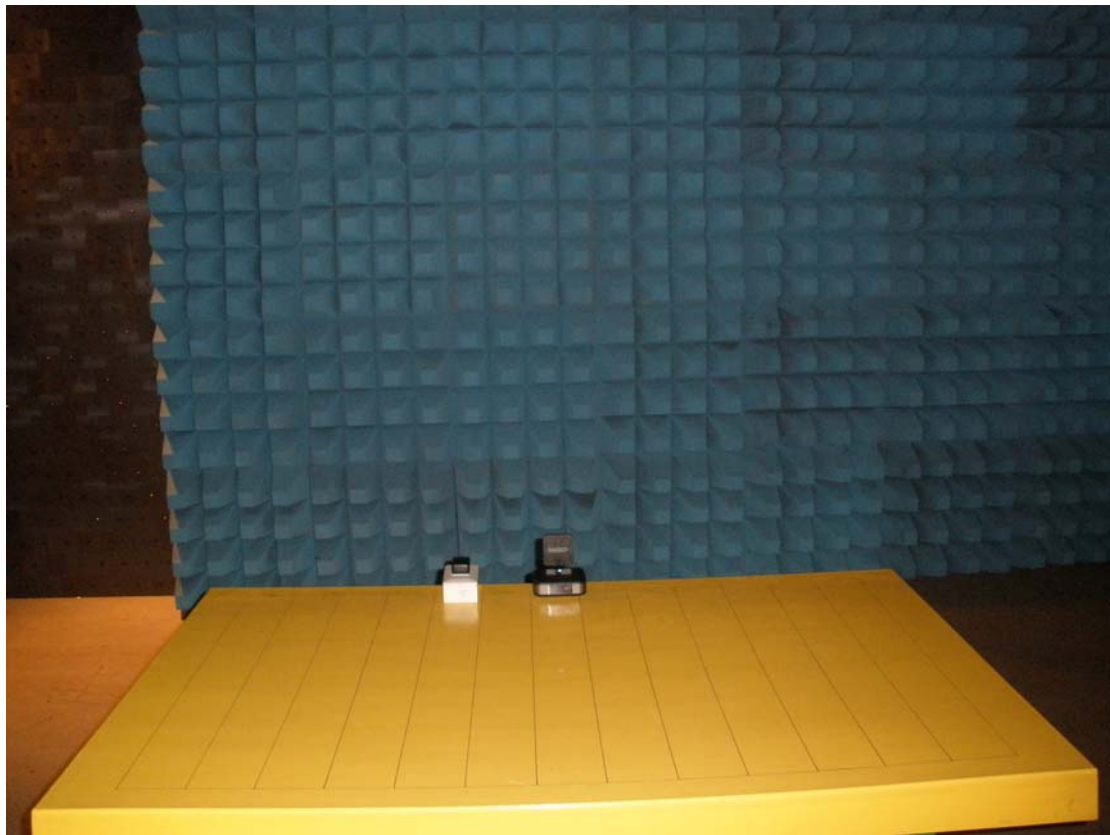
Radiated Emission Test set-up photo
