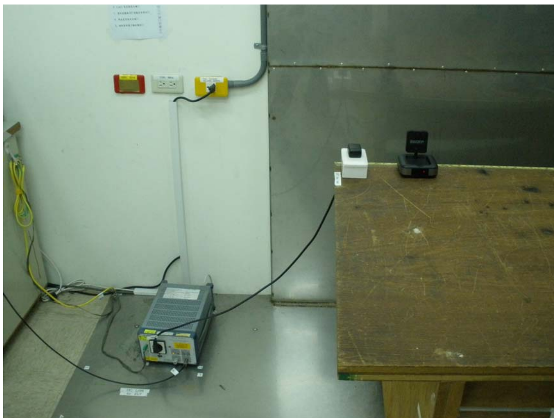
Conducted Emission Test Set-up photo
