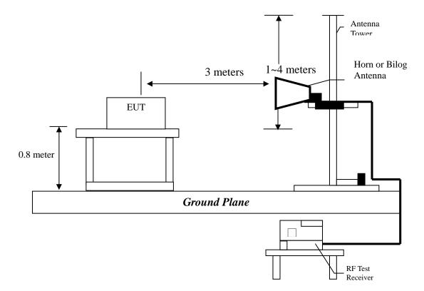
The signal is maximized through rotation and placement in the three orthogonal axes. Radiated emission measurements were performed from 30 MHz to 25 GHz. Spectrum Analyzer Resolution Bandwidth is 100 kHz or greater for frequencies 30 MHz to 1 GHz, 1MHz – for frequencies above 1 GHz.
