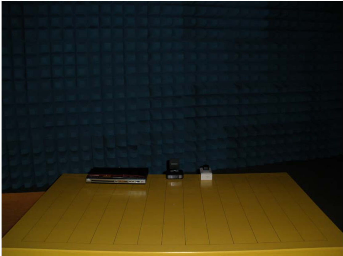
Radiated Emission Test set-up photo
