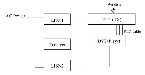
The EUT are connected to the main power through a line impedance stabilization network (LISN). This provides a 50 ohm/50uH coupling impedance for the measuring equipment. The peripheral devices are also connected to the main power through a LISN that provides a 50ohm/50uH coupling impedance with 50ohm termination.
