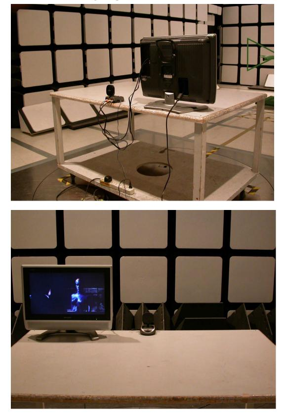
Photos of Conduction Measuring Setup
