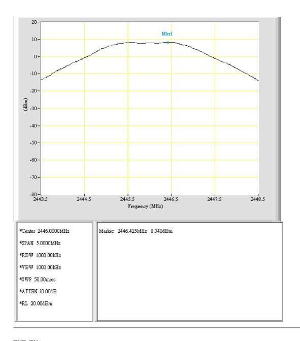
Purpose: Output\_Pwr Condition: CH5
