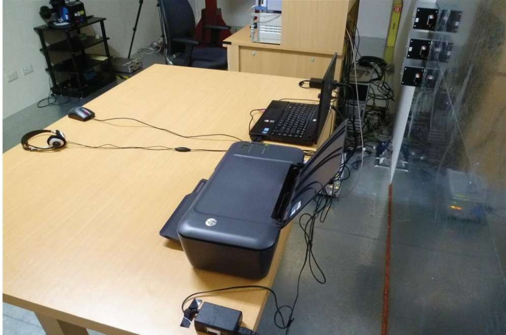
Photograph 5: Set-up for for Mains Conducted testing Back
