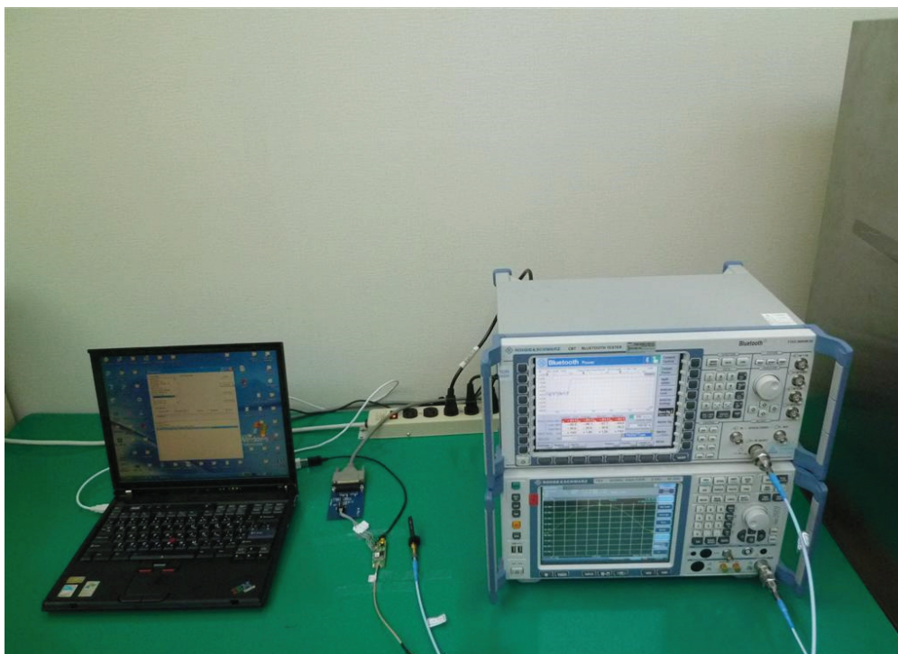
Photograph 4: Set-up for Conducted testing
