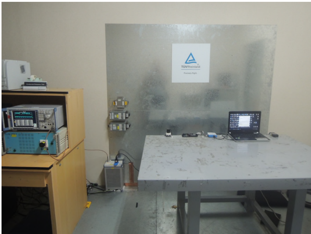
Photograph 6: Set-up for Mains Conducted testing Front
