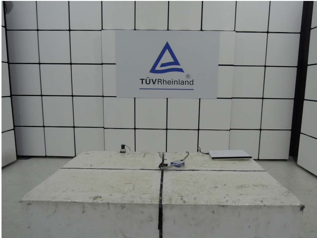
Photograph 2: Set-up for Spurious Emissions (Back View 1)
