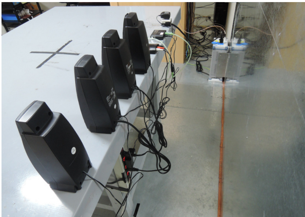
Photograph 5: Set-up for for Mains Conducted testing Back
