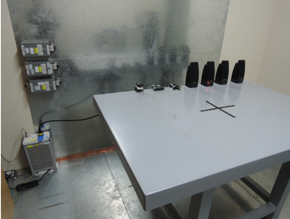
Photograph 6: Set-up for for Mains Conducted testing Front
