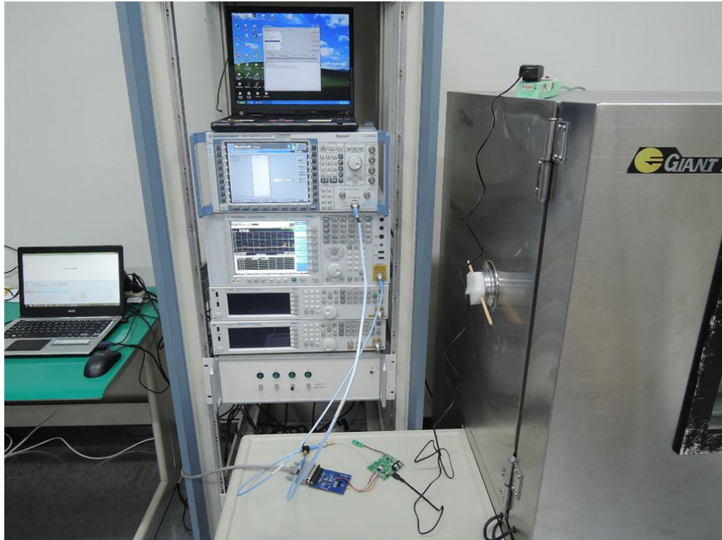
Photograph 4: Set-up for Conducted testing
