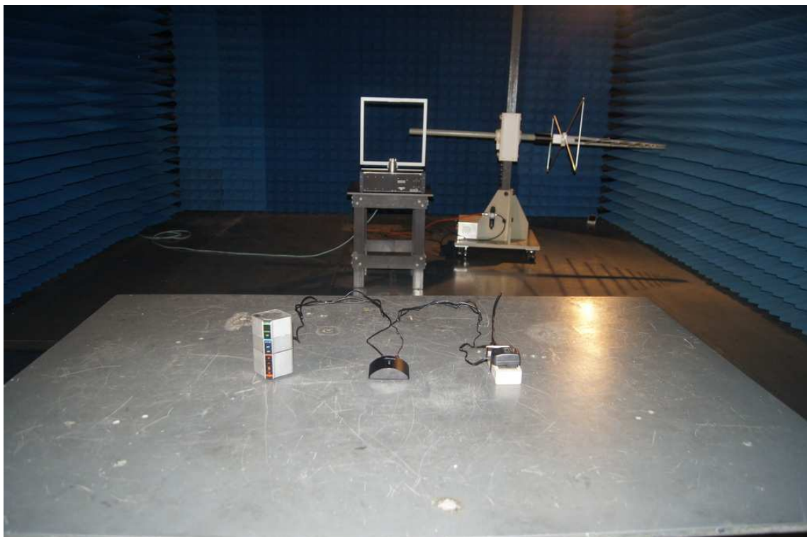
Photograph 2: Set-up for Spurious Emissions (9kHz-30MHz)
