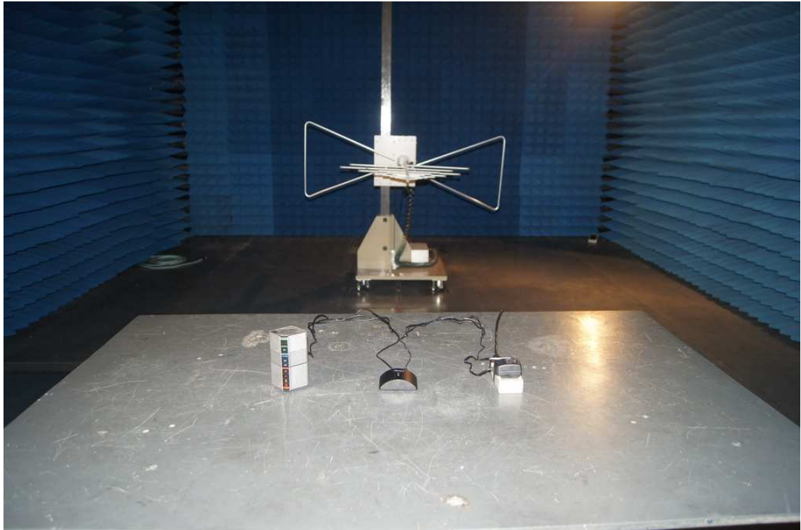
Photograph 4: Set-up for Spurious Emissions (1GHz-18GHz)
