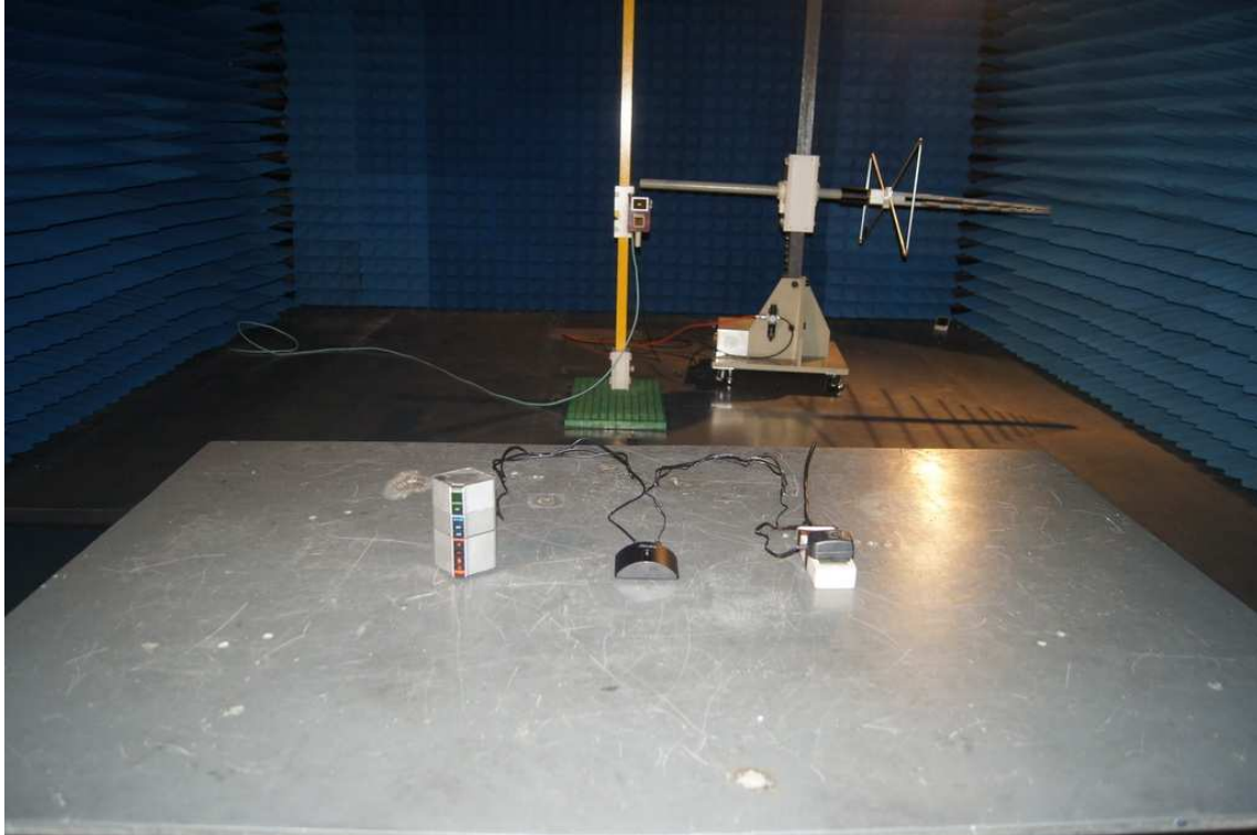
Photograph 5: Set-up for Spurious Emissions (18GHz-26GHz)
