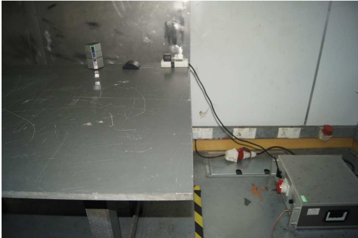
Photograph 2: Set-up for Spurious Emissions (9kHz-30MHz)
