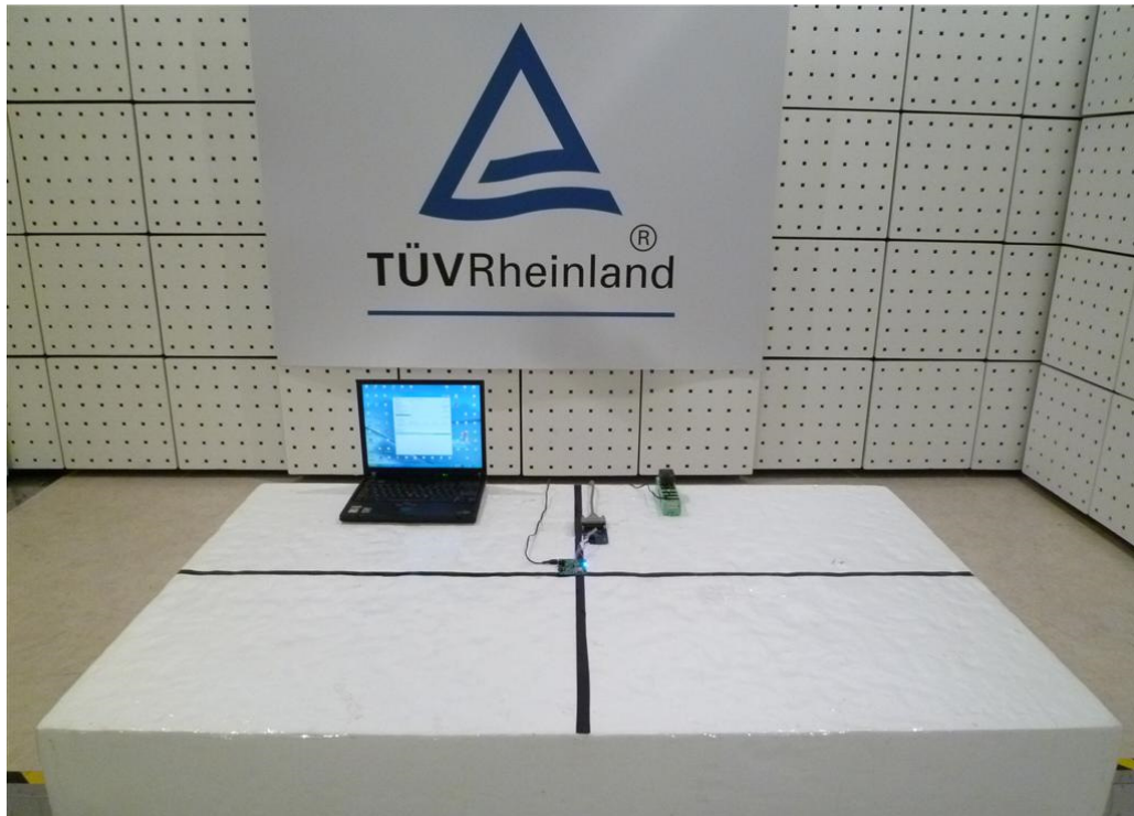
Photograph 1: Set-up for Spurious Emissions (Front View)
