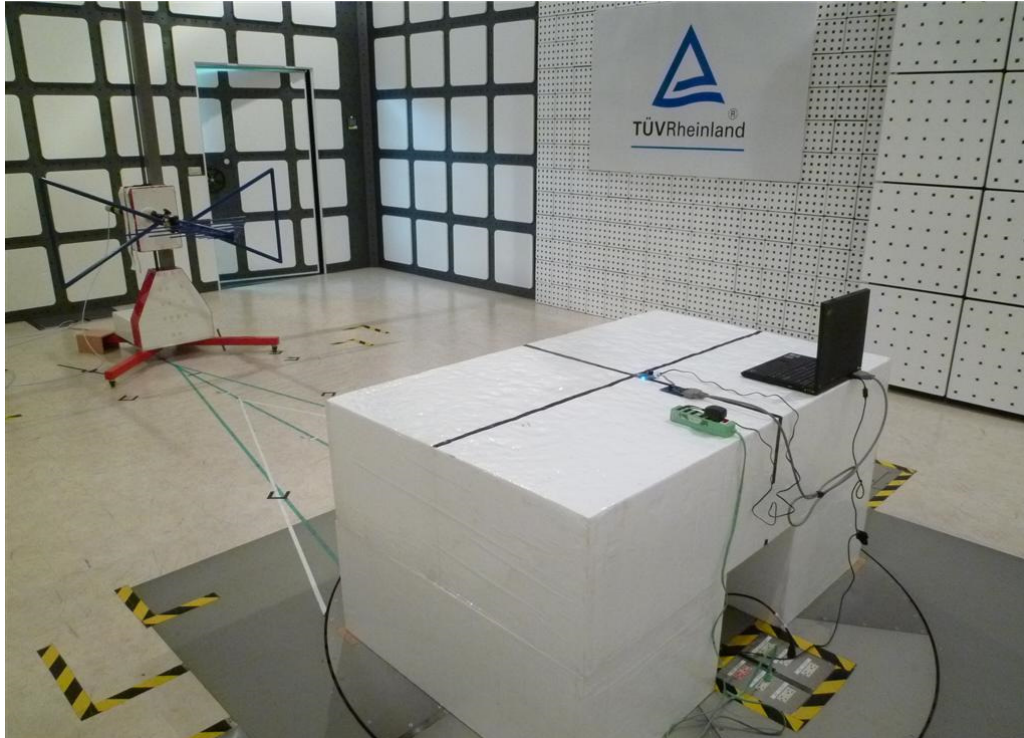
Photograph 2: Set-up for Spurious Emissions (Back View 1)
