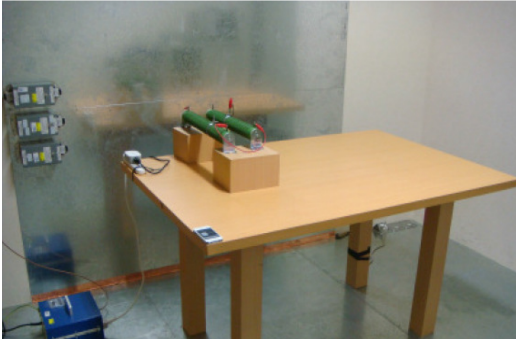
Photograph 5: Set-up for for Mains Conducted testing Back
