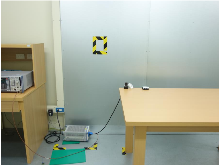
Photograph 7: Set-up for AC Mains (Front View)
