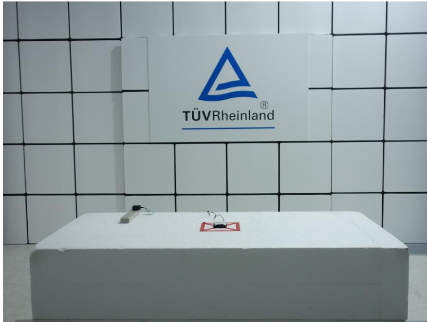
Photograph 9: Set-up for Spurious Emissions (Front View 1)
