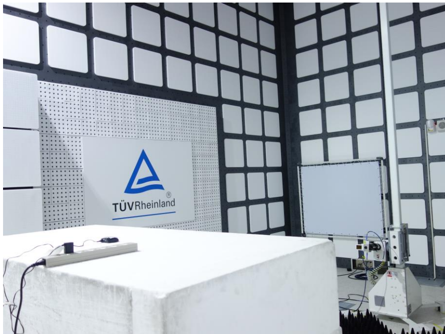
Photograph 6: Set-up for Spurious Emissions (Back View 4)
