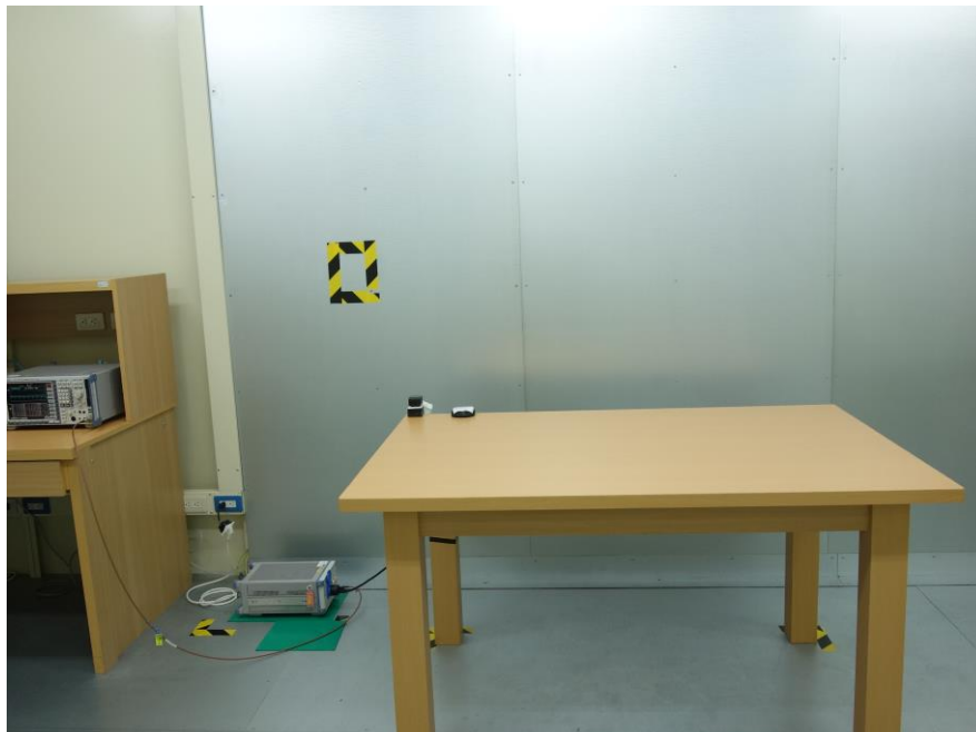
Photograph 12: Set-up for AC Mains (Front View)
