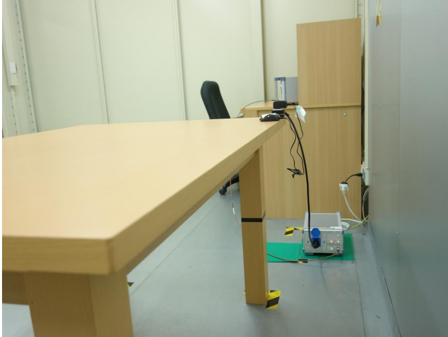
Photograph 13: Set-up for AC Mains (Back View)
