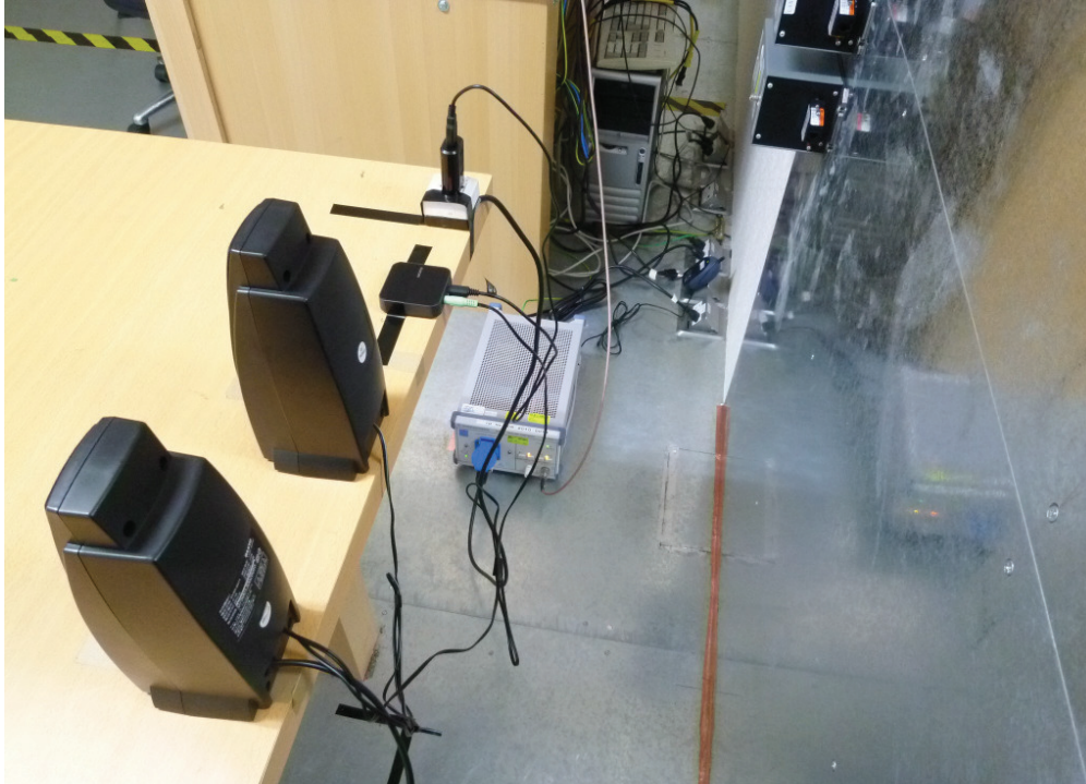
Photograph 5: Set-up for for Mains Conducted testing Back
