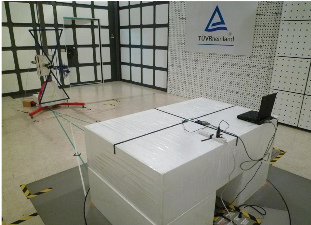
Photograph 2: Set-up for Spurious Emissions (Back View 1)
