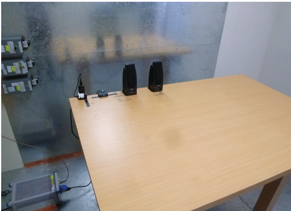
Photograph 6: Set-up for for Mains Conducted testing Front
