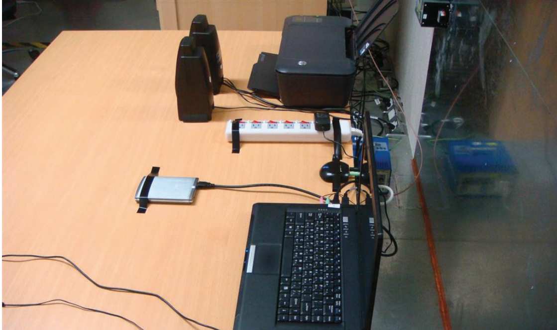
Photograph 5: Set-up for for Mains Conducted testing Back
