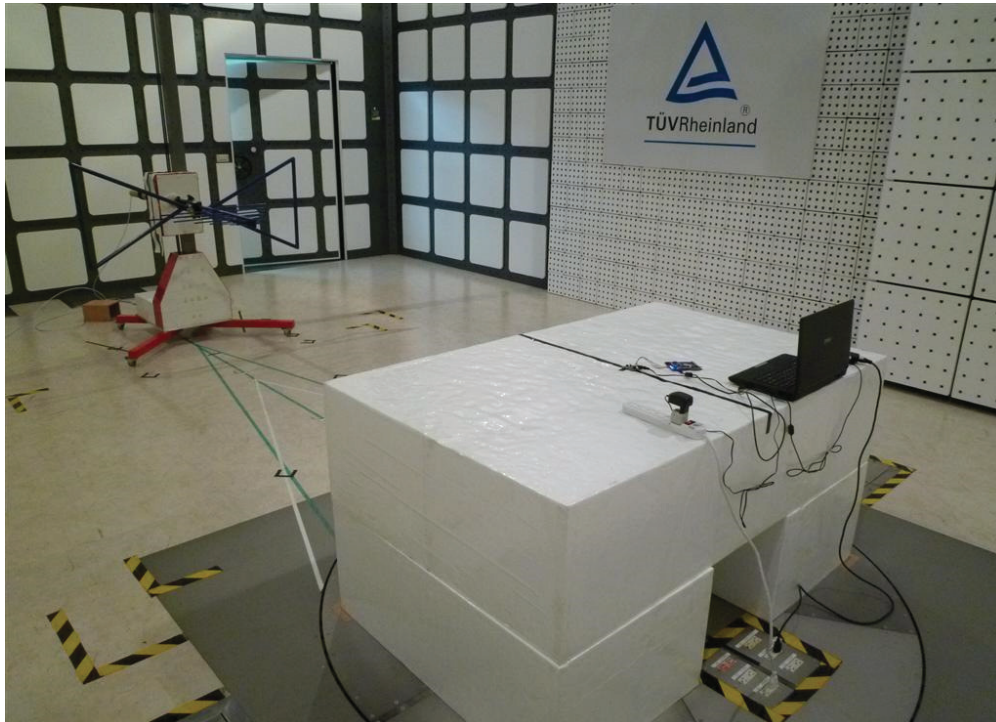
Photograph 2: Set-up for Spurious Emissions (Back View 1)
