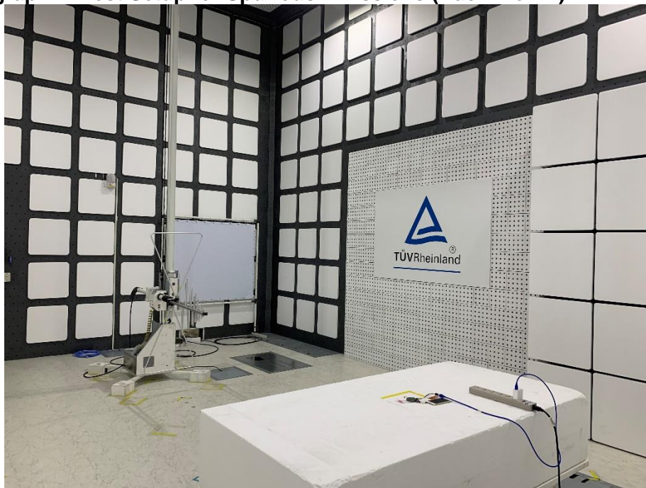
Photograph 4: Test Setup for Spurious Emissions (Back View 2)
