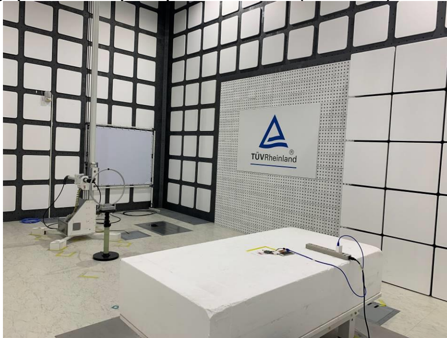
Photograph 4: Test Setup for Spurious Emissions (Back View 2)
