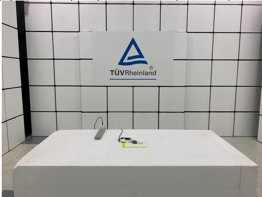
Photograph 2: Test Setup for Spurious Emissions (Front View 2)
