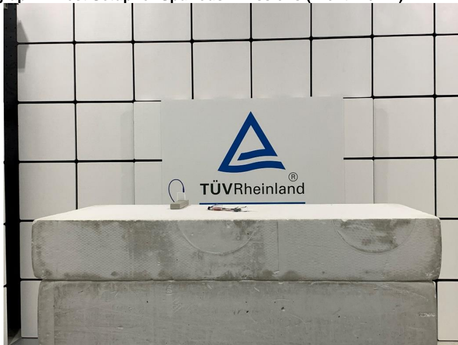
Photograph 2: Test Setup for Spurious Emissions (Front View 2)
